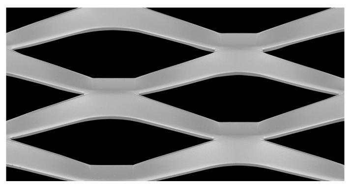
LW Pitch:135.00mmStrand Width:15.00mmSW Pitch:48.00mmThickness:3.00mmWeight:5.06 kg / m2Open Area:37%
